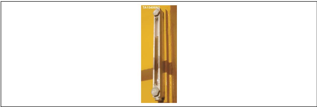
Figure 6. Hydraulic reservoir sight glass
