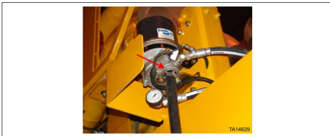
Figure 5. Discharge line unloader (DLU) valve
