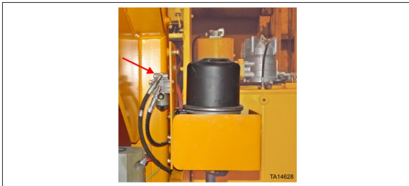
Figure 4. Location of compressor governor
